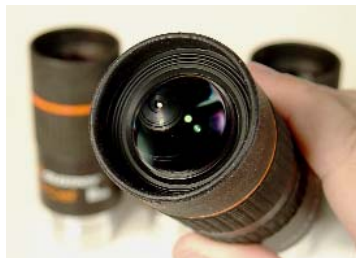
EYE TO THE SKY: Each X-Cel eyepiece (2.3mm shown) has a wide-field lens with 20 millimetres of eye relief, making it easy to look through even the highest-power models. No squinting through these or brushing the eyepiece with your eyelashes and sneaking the lens. And no worries about getting too close to a metal eyepiece top on cold winter nights. Once you use long-eye-relief eyepieces like the X-Cels, you may never return to conventional models.
