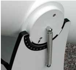
Top left: The primary 8-inch mirror is supported at its edge, which leaves the back of the mirror itself exposed (that's its reflection at the rear of the tube). The numbered dials are mostly for show and have little practical application. Above left: When an eyepiece is inserted or extracted from the focuser, the springs on the mount provide enough tension to prevent the tube from tipping up or down as the balance point varies.
