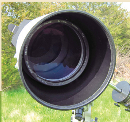
DARK GLASS A 6-inch objective lens (left) is an impressive optic by any standard. Three baffles within the tube suppress stray light. A welcome feature with this telescope is the heavy-duty 3-inch-diameter focuser assembly with 10-to-1 fine-focus reduction—a very solid and smoothly functioning unit for an instrument at this price point.
