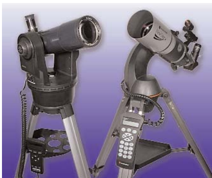
NEW OPTIONS: Relatively low-cost "Go To" telescopes, such as the Meade ETX70-AT (left) and the Celestron NexStar 80, offer computerized finding of sky objects.
